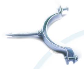
CTECH Nail Clamp have been designed keeping in view the concrete wall where this clamps make a solid grip .open the clamp place pipe in a such a way that the rod align with clamp. Close clamp and tighten the nut bolt.
